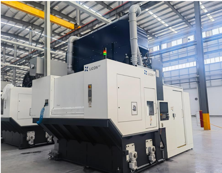
2023-07-17-Tuopu-5.jpg One of the 29 LiFLEX I 12126 machining centres purchased from Tuopu.
