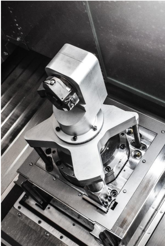
2023-06-09-Haldex-LiFLEX-II-766-i-DL-B2-Spindel.jpg 用于铣削的坚固角度头
