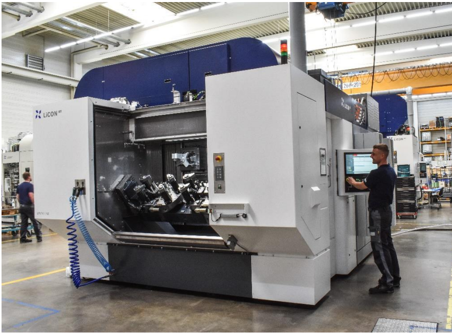
2023-06-09-Haldex-LiFLEX-II-766-i-DL-B2-Maschine+Bediener-1.jpg Twin spindle machining center LiFLEX II 766 i DL B2 with operator
