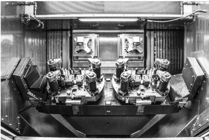
2023-06-09-Haldex-LiFLEX-II-766-i-DL-B2-Innenraum.jpg LiFLEX II 766 i DL B2 machining area with clamping fixtures for calipers
