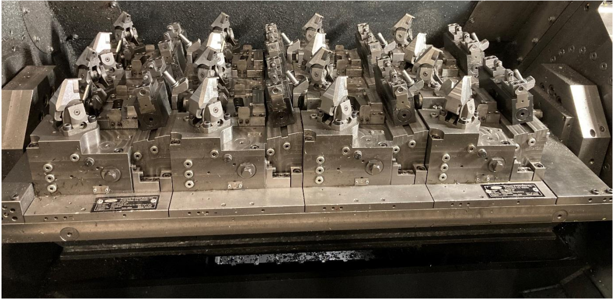
LiCON-Success-Story-Celikform-3.jpg Clamping device for door hinges
